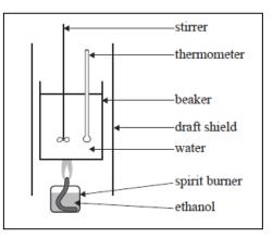
ii. Why is the result only an estimate and not an accurate measure of the total energy released? *The equipment is poorly insulated and hence a great deal of energy is not absorbed by the water but is lost to the surroundings.*
